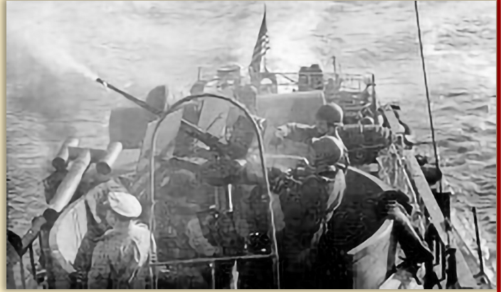
The number two 20mm gun crew of LCI(L) 85 at anti-aircraft practice (Note the "Charlie Noble" smoke exhaust stack disassembled to give a free field of fire)
