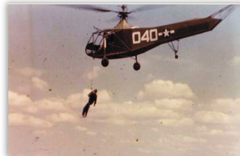
Coast Guard hoist demonstration from the HNS-1 in 1944 (U.S. Coast Guard Photo)
