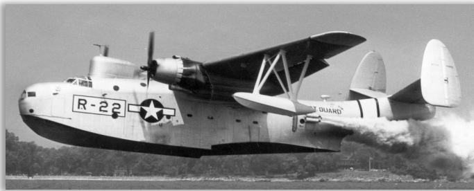
A Coast Guard Martin PBM-5G Mariner seaplane performing a JATO assisted takeoff.
