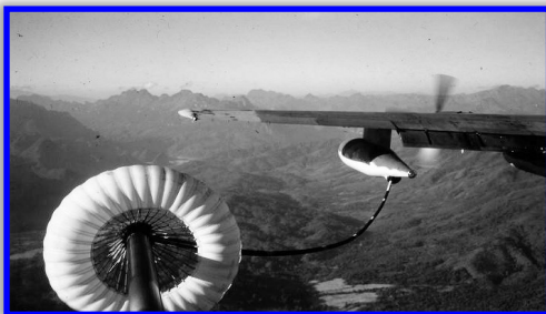
HH-3E pilot's view from his helicopter "plugged into" a HC- 130P tanker
