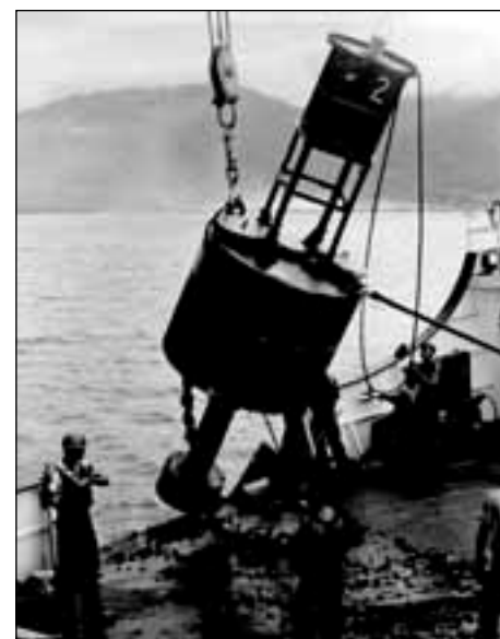
A 6,000-lb. harbor entrance buoy is hoisted aboard CGC Blackhaw (WLB-390) near Black Rock Quarry, southeast of Danang in 1970.
